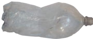
**5. Bottle Worn, Cracked or Damaged** - Replace with a new plastic 2-liter bottle that previously held fizzy pop. You can't repair these. Don't use a water bottle because they aren't strong enough to hold the pressure.
