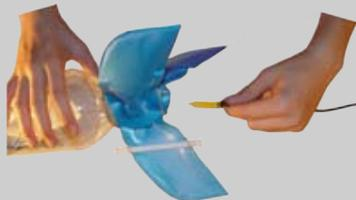
Push the yellow bulb on one end of the launcher hose into the nozzle cap. Now the water won't leak out.
