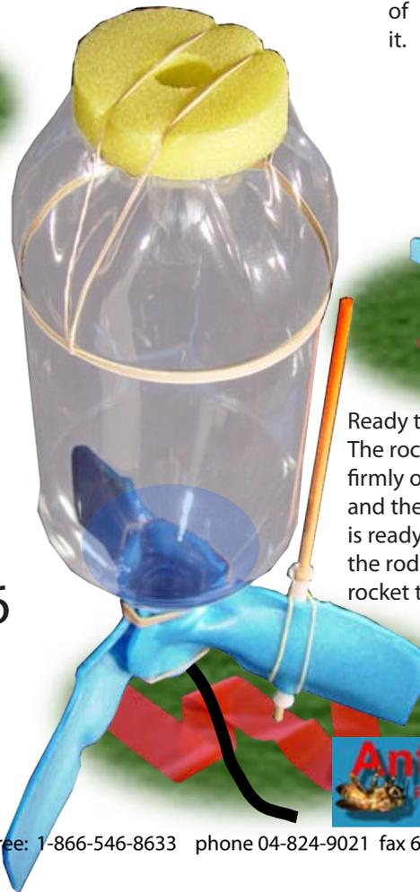
Ready to fill with air! The rocket's fins rest firmly on the ground and the guide tube is ready to slide up the rod when the rocket takes off.
