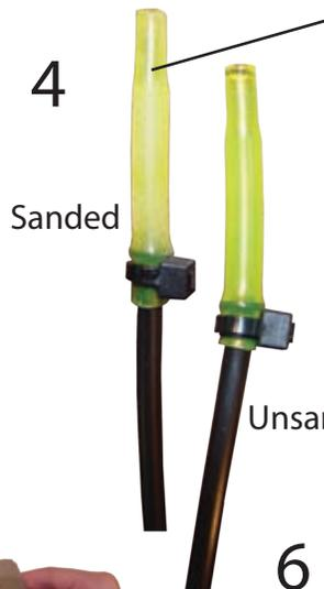
This is what the bulb looks like when it is properly modified. Notice how the surface is not as shiny as the unsanded bulb.
