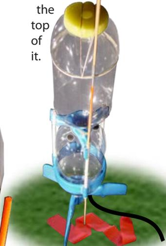
6 Ready to fill with air! The rocket's fins rest firmly on the ground and the guide tube is ready to slide up the rod when the rocket takes off.
