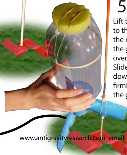
5 Lift the rocket to the top of the rod and slide the guide tube over the rod. Slide the rocket down until it rests firmly on its fins on the ground.
